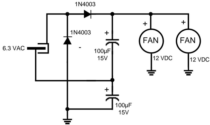
Figure 5 – Voltage Doubler Circuit
